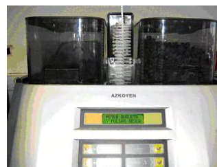
Cleaning supply tube, insert brush to the bottom.
